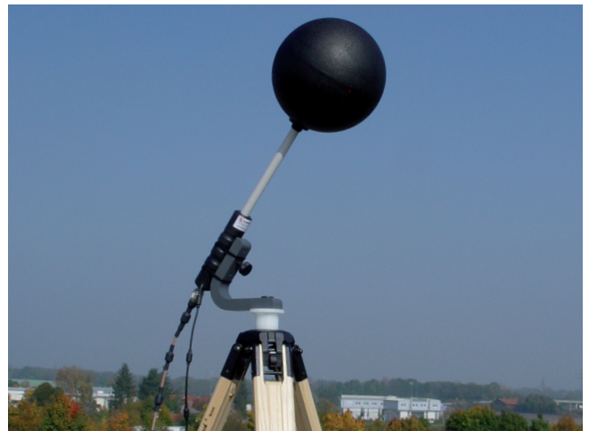
The 9102 or 9103 with the 9171 Isotropic Antenna is a comfortable test solution for immission measurements.
